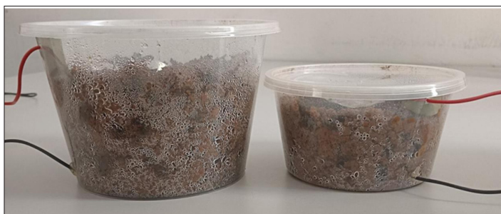
Figure 2. 700 ml and 350 ml MFC chambers
